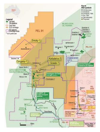
The Hanson-1 discovery well was completed on 23 January 2012, and was perforated across 2.7 metres of the McKinlay Formation. The well was then flow-tested for one hour, with initial production measured at a rate of 763 bopd.
