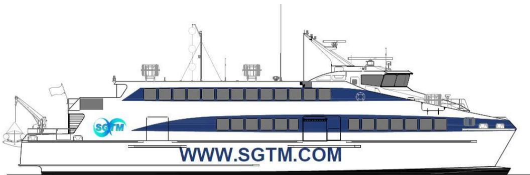
***The Passenger Express 41 to be constructed by Austal's shipyard in Vietnam will accommodate 400 passengers and 20 tonnes of cargo over 2 decks. (Image: Austal)***
