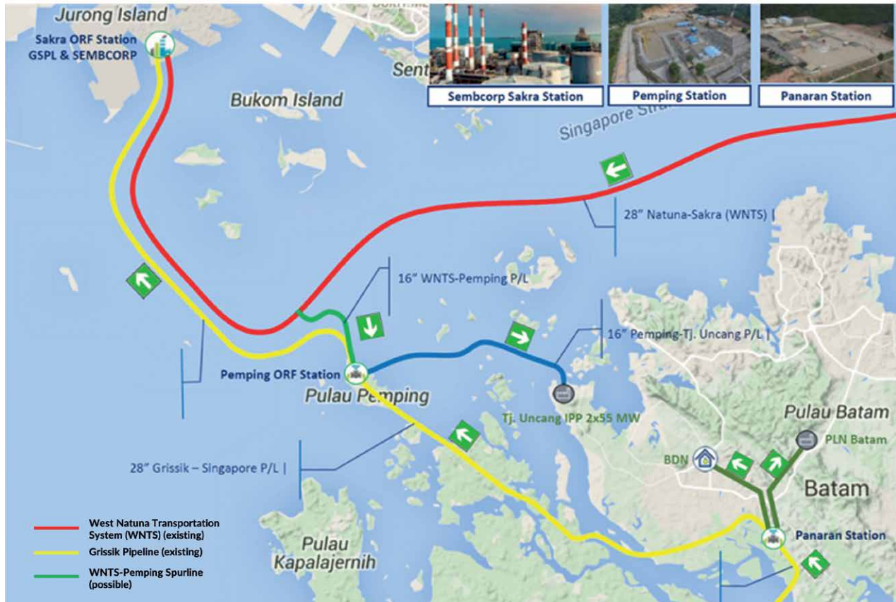
Figure 2.5.7: Illustration of the southern approaches of the West Natuna Transportation System and its connection to Singapore
