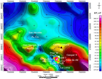
Aeromagnetic Survey El Pilar
