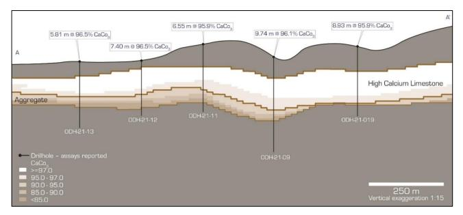
Figure 1: Cross section A - A' highlighting the thickness and continuity of grade across the MRE model.
