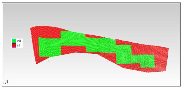
Figure 11: Quartz Hill Classification (Oblique Long Section View Facing 165°)
