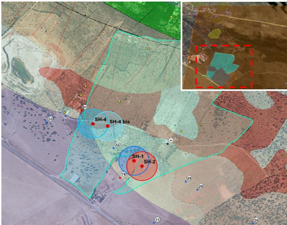
Figure 3: New water bore drill hole locations within proposed plant and TSF area showing 100m perimeter of influence around each bore hole (inset – location within Company tenement, see legend below)
