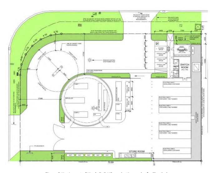
Figure 2 Key Layout of Lion's PoB H2 production and refuelling hub
