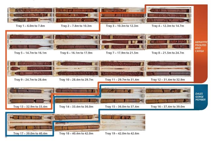
Figure 2: Diamond drill hole METDD00171 highlighting hematitic loose and pisolitic detritals, canga and Dales Gorge Member
