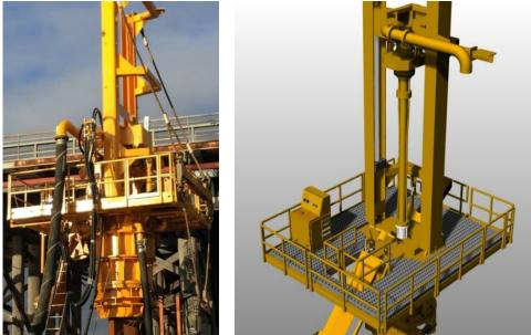
Figure 27: Pile top drill rig used for DDD pile installation
