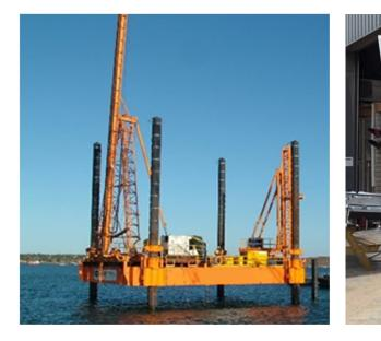
Figure 20: SEMP used to install mooring piles.
