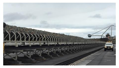
Figure 35: Concept conveyor on footings feeding radial shiploader to TSV
