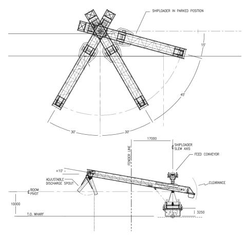
Figure 23: Typical radial shiploader for barge loading
