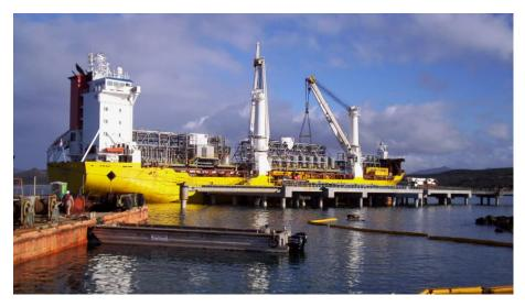
Figure 30: HLS transporting prefabricated modules
