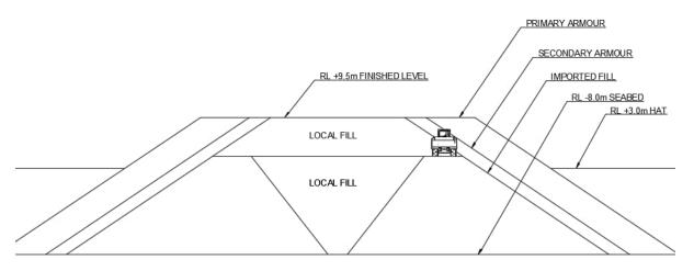
Figure 12: Assumed cross section of rock wharf illustrating proposed construction methodology
