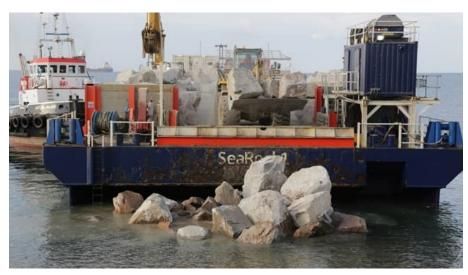
Figure 14: Typical rock barge being offloaded by front-end loader
