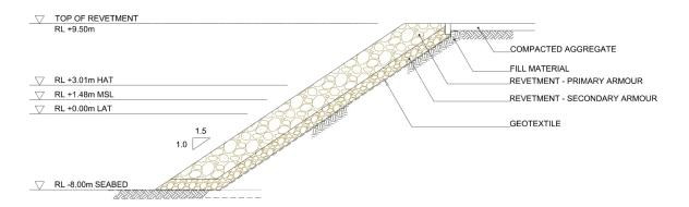
Figure 11: Assumed cross section of wharf construction showing fill and armour
