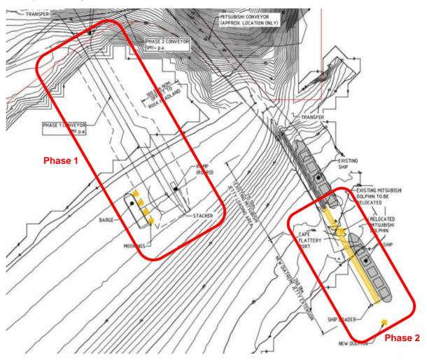
Figure 2: Site plan and general overview of phased construction approach
