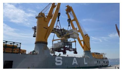
Figure 36: HLS lifting a fully assembled shiploader
