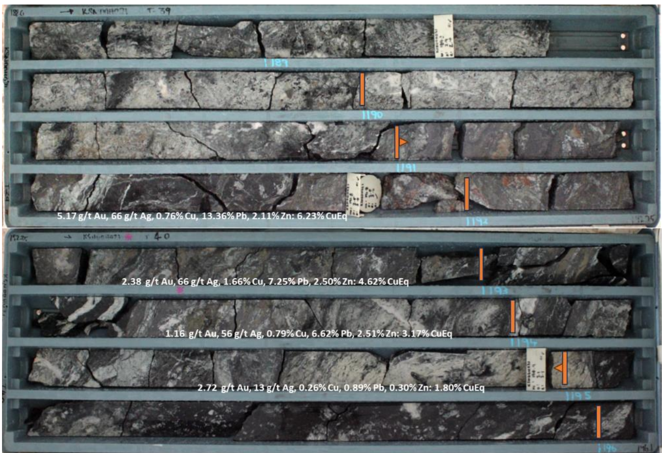
Figure 3: Drill core from KSNDDH021 (4m wide sulphide rich breccia lode (estimated true width of 2m) within a broader 31.6m wide brecciated and veined lode zone from 175.3mdh).
