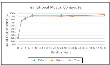
Figure 6. Gravity Gold + Cyanide Leach Curves for Transitional composites
