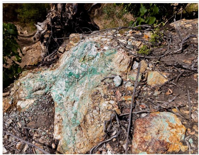
Figure 1. Outcropping high-grade copper mineralisation associated with magmatic quartz bodies within Briggs Central
