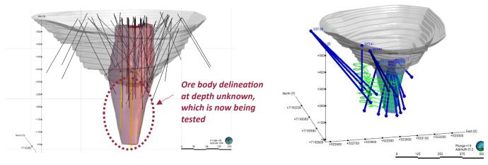
Figure 1 - Historic delineation drill holes (black) and completed reverse circulation drill holes (orange). Note the lack of pierce points at depth to adequately model the size of the Sable kimberlite pipe.
