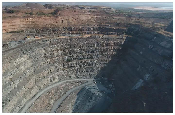
Figure 4: Syama Open Pit with 1,200mRL mid-pit portal in centre right of photo
