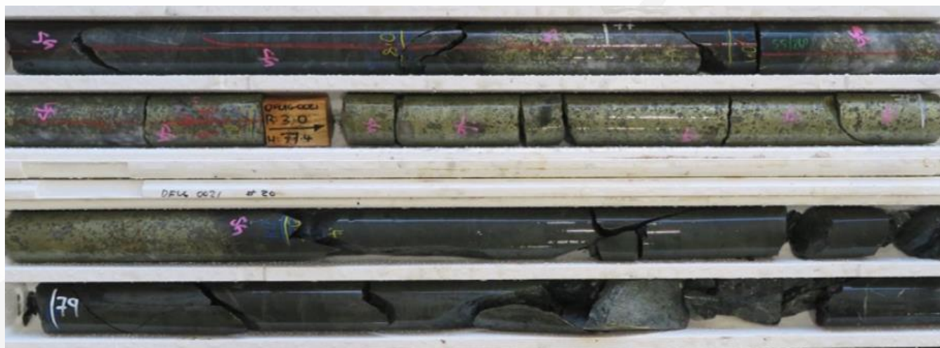
Figure 3. Da Vinci intersection, DFUG0021 - 1.6m @ 143.8g/t Au and 17.8% Cu from 76.8mdh
