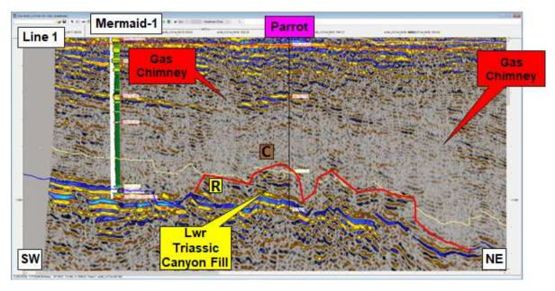
Seismic cross section of the Parrot prospect with seismic evidence of gas chimneys on either side of prospect
