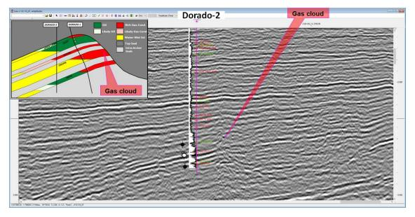
Seismic cross section across Dorado with gas cloud associated with up-dip gas accumulation
