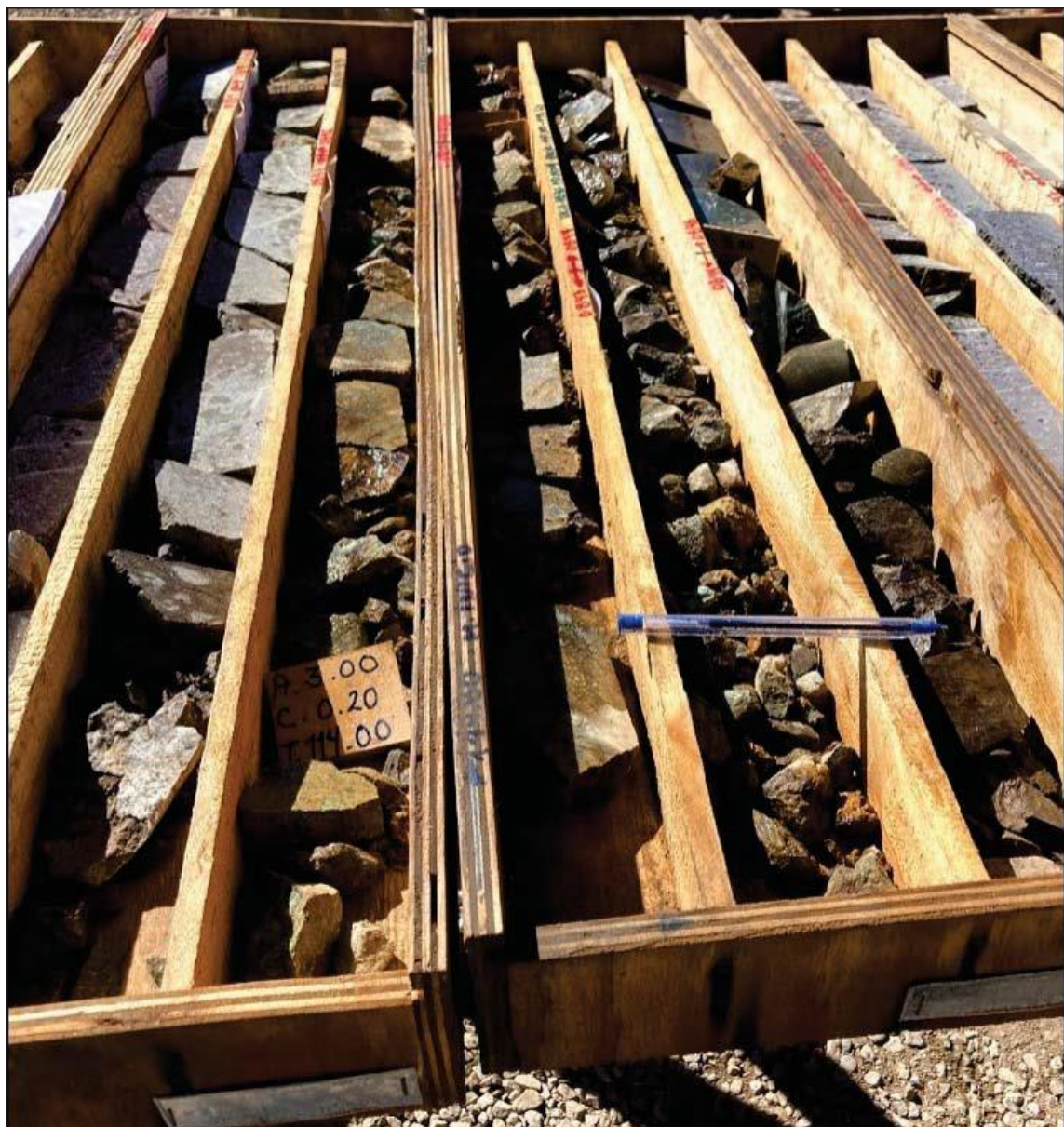
Figure 2.13: Core boxes showing metallic labels, core blocks and sampling intervals (red pen)
