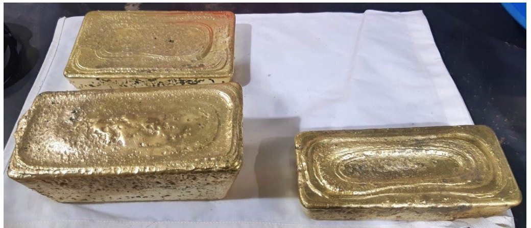
Figure 1: CIL Bars on the left and latest gravity bar on the right from Warrawoona
