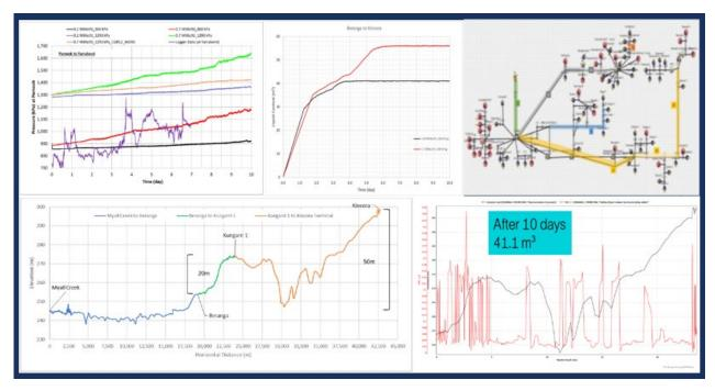
Examples of SLB dynamic gathering system modelling calculating liquid hold up
