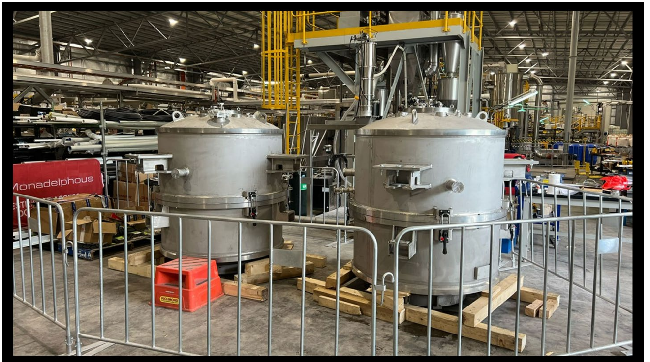
Sapphire grower shells, delivered and ready for installation
