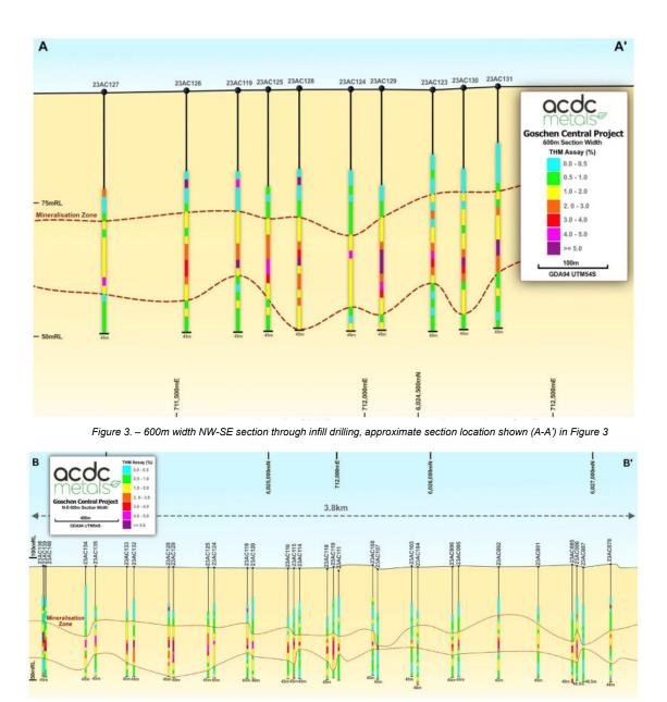
Figure 4. – NS section through infill drilling, Section location shown (B-B') in Figure 3
