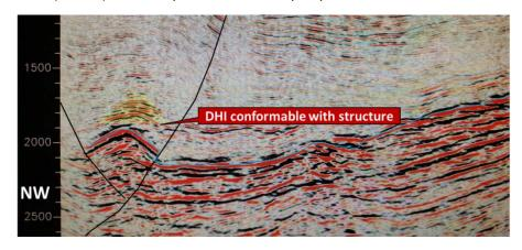
Figure 1: 2D Seismic section through an anticline with bright seismic events (yellow highlights) over the closure area, indicating potentially gas charged reservoir sandstones
