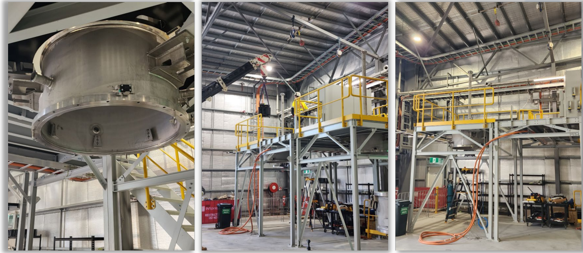
Assembly of the first 2 (Phase A) sapphire growth units at final stages
