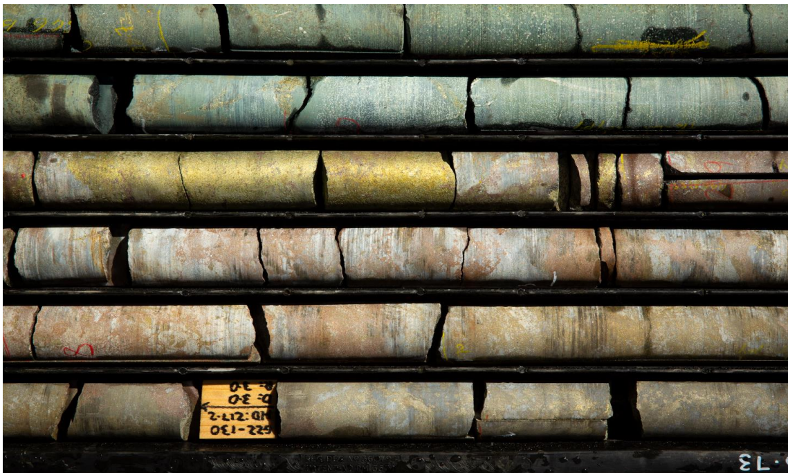
Drill core samples from Xantho Extended showing massive chalcopyrite, and sub-massive sphalerite and pyrite.
