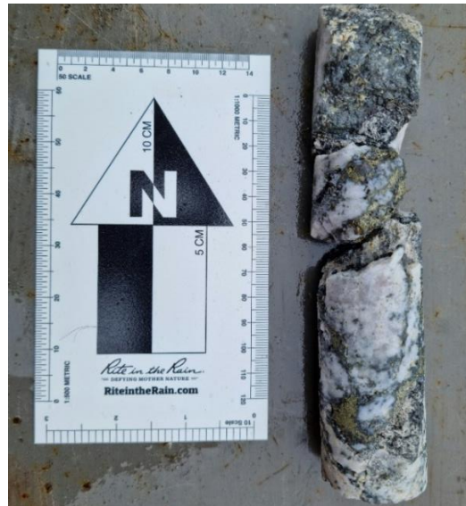
Drone based magnetics survey at Cutters (LHS). Example of vein style mineralisation intersected using portable small drills. Quartz Carbonate Vein hosting chalcopyrite and pyrite mineralisation (RHS).
