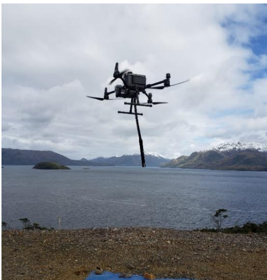
Drone based magnetics survey at Cutters (LHS). Example of vein style mineralisation intersected using portable small drills. Quartz Carbonate Vein hosting chalcopyrite and pyrite mineralisation (RHS).
