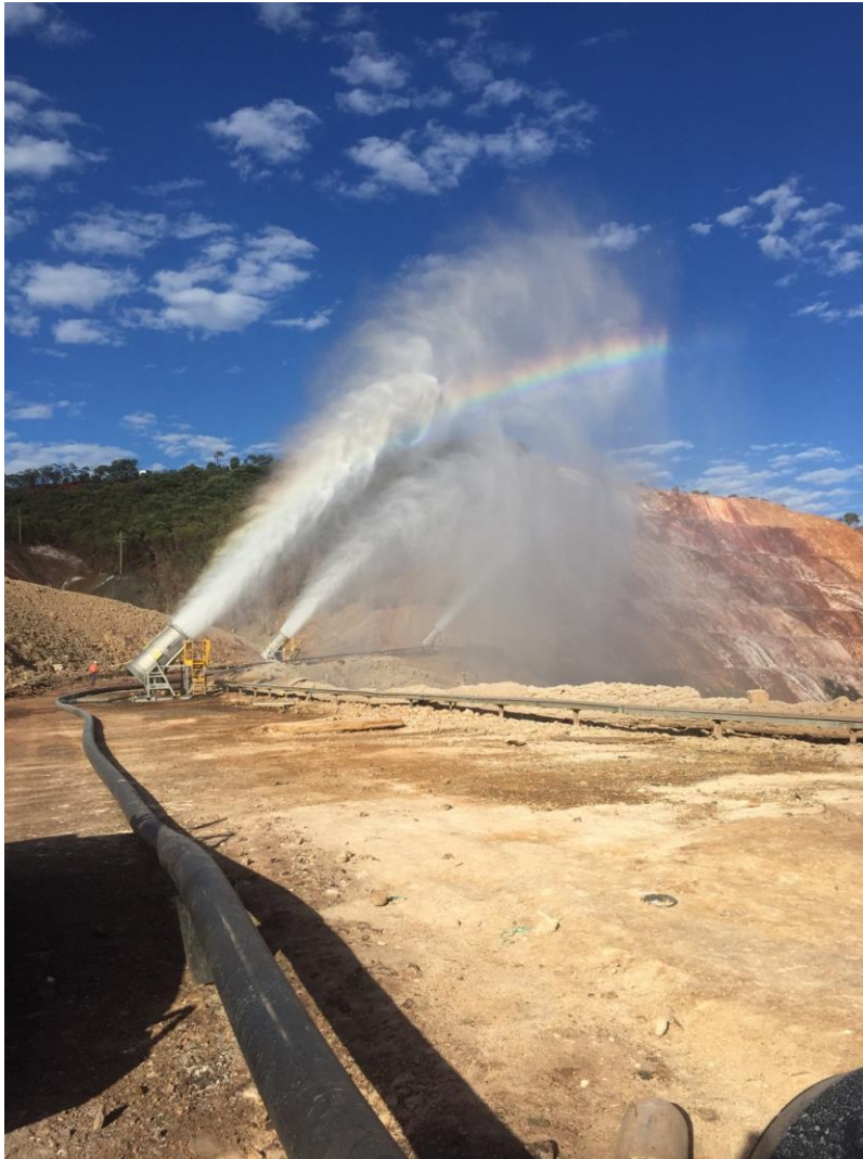
New high-efficiency mechanical evaporators in operation at the EPit at Capricorn Copper during the Dec-Qtr.
